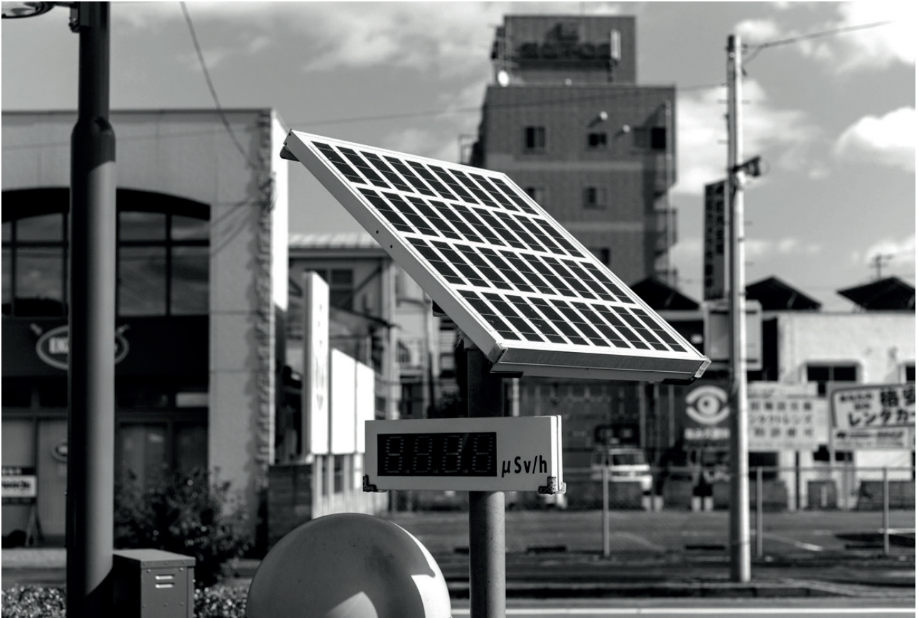
A solar-powered Geiger counter at Namie station.
